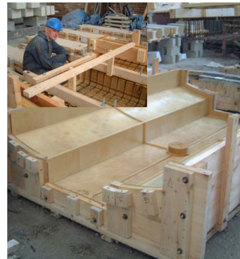
3 No. 12m long suspended walkways were also manufactured in sections for use in the atrium inside the building. The thickness of these units was 75mm and incorporated lighting voids.
