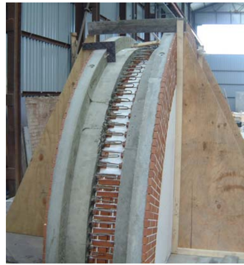
Double faced colonnade arches were manufactured as in two separate sections and then stitched together on a jig, holding the soffit bricks in place
