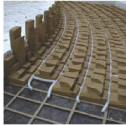
Each brick header is dovetailed. A grid is laid out on the base of the mould to ensure accurate spacing of the bricks.
