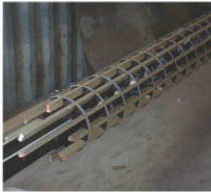
The plug for the fibreglass mould was made in-house using a steel core and decreasing timber loftings to create the taper.
