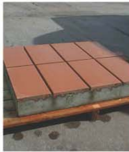
Sample panels were manufactured for architectural approval and to check that the keyed profile on the back of tiles was acceptable.
