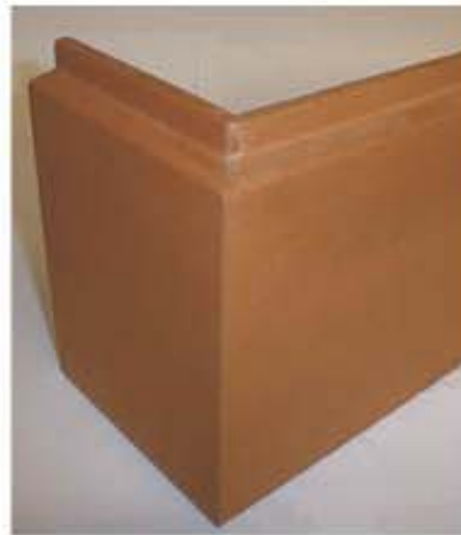
50% of all pieces supplied were corner returns. These were manufactured from standard tiles by water jet cutting mitres and fabricating back together with epoxy resin.
